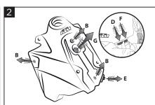
Remove seat screw (B) and the screws on the side. Remove the tank screw (G), then empty any remaining fuel from the tank. Remove the (D/E/F) fasteners and remove the fuel pump.
