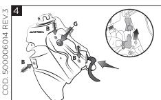
Place the Acerbis fuel tank (A) on the bike. Insert the tank and seat screws (G/B) as indicated in the diagram.
