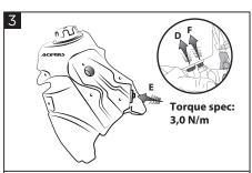
On the fuel tank Acerbis (A), reconnect the fuel pump (E) with the original screws/hardware.
