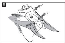
Assemble the radiator scoops with the screws (C).
